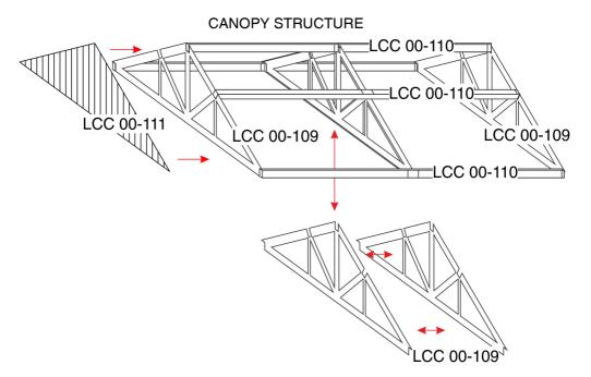
Start by gluing two LCC 00-109 together. Glue LCC 00-111 to one of the single LCC 00-109 elements. Ensure that the parts are flush with each other at the top. Using LCC 00-110 strips glue LCC 00-109 together to form the internal structure of the canopy. Use the markings in the middle of LCC 00-110 to alight the doubled up LCC 00-109. Because LCC 00-110 have been shortened only on one side make sure LCC 00-110 are facing in the same direction to ensure correct alignment.
